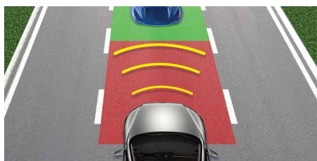
Forward Collision Warning System (FCWS) to keep a safe distance
